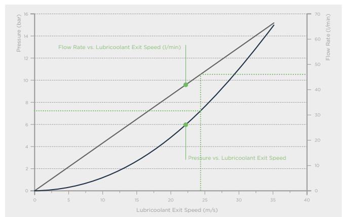
Starting from the pressure, you can directly find the associated lubricoolant exit speed. The grey line shows the correlation between the lubricoolant exit speed and associated lubricoolant flow rate.
